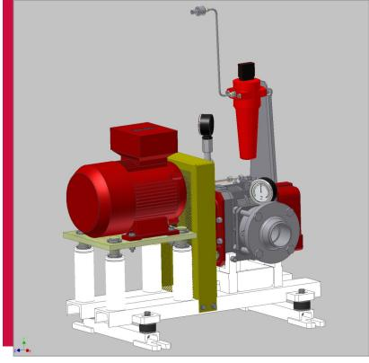
View from the discharge side with an analog thermometer of gas in the discharge pipe.
